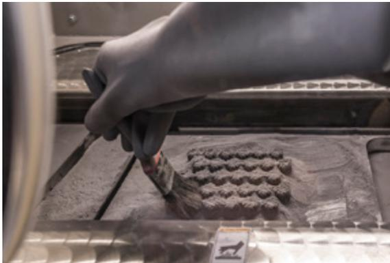
Precision metal sintering machines build production-quality parts in metals like stainless steel, cobalt chrome, aluminum and others.
