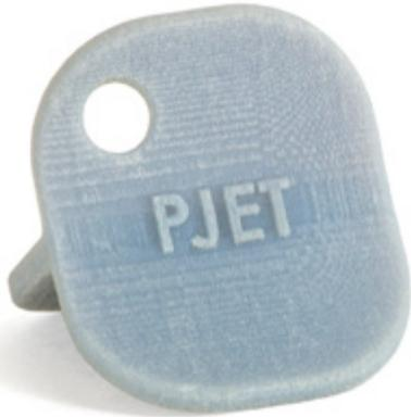
**PolyJet (PJET)** uses a print head to spray layers of photopolymer resin that are cured, one after another, using ultraviolet light. The layers are very thin allowing superior resolution. The material is supported by gel matrix that is removed after completion of the part.
