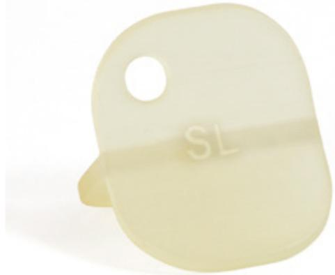
**Stereolithography (SL)** uses a computer controlled laser to build parts in a pool of UV-curable resin. As each layer is drawn by the laser, the part is lowered in the pool of liquid resin allowing the next layer of liquid to be solidified. Quality of the finished part depends largely on the quality of the equipment and process used.
