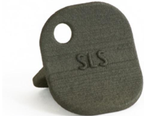
**Selective laser sintering (SLS)** employs a computer controlled CO<sub>2</sub> laser to fuse layers of powdered material such as nylon from the bottom up. Strength is better than that of SL but lower than that produced by subtractive processes like injection molding or CNC machining. It also has some use as a production method.
