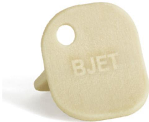
**Binder jetting** is one of the simplest and most basic additive prototyping processes. An inkjet print head moves across a bed of powder, selectively depositing a liquid binding material, and the process is repeated until the complete part has been formed. After completion, the unbound powder is removed leaving the finished object.
